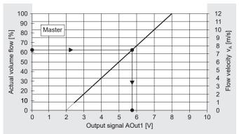
The operation modes 2-8 V are set at the **Master** and **Slave**. The Master is set to  $\mathbf{OVF_{min}} = 35\%$  V<sub>max</sub> and  $\mathbf{OVF_{max}} = 70\%$  V<sub>max</sub> and activated with U = 2 to 8 V. When U = 6.7 V, according to page 4, formula [3]:
