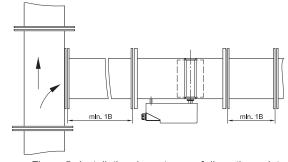
Figure 5: Installation downstream of disruption point, e.g. T-pieces
