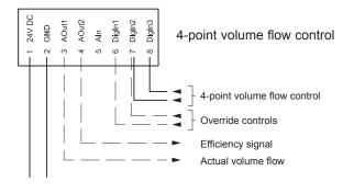
: Connections are absolutely required.: Connections are optional.
