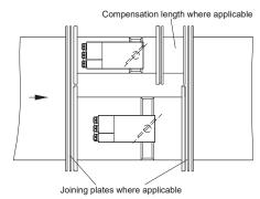
Figure 6: Installation in double arrangement
