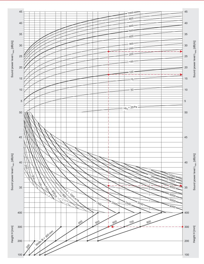
In the above nomogram, the sound power level inside the connecting duct is dimensioned as an overall level  $L_{WA}$ . Octave sound power levels  $L_{W-Oct}$  for every size and any required operating point are obtained from the WILDEBOER dimensioning software.
