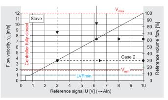
If the actual volume flow at the Master does not reach the reference volume flow, the Slave follows the actual volume flow!  $\Rightarrow$  see example 2!
