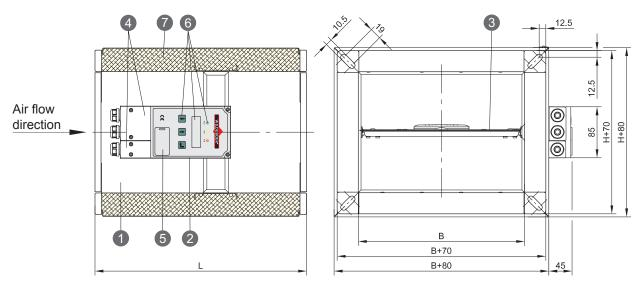
**VKE1 volume flow controllers** are maintenance-free, electronic controllers that produce constant and variable volume flows in ventilation and air conditioning systems.
