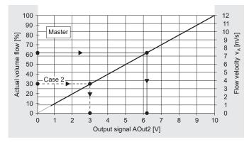
The operation modes 0-10 V are set at the **Master** and **Slave**. The Master is then controlled with U = 0 to 10 V. For **OVF**<sub>min</sub> = 35% V<sub>max</sub> and **OVF**<sub>max</sub> = 70% V<sub>max</sub> as well as with e.g. U = 7.6 V according to page 4, formula [1]: V<sub>ref</sub> =  $35\% + (70\% - 35\%) \cdot 7.6 \text{ V} : 10 \text{ V} = 62\% \text{ V}_{max}$
