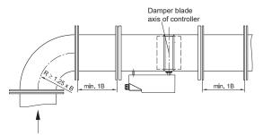
Figure 4: Installation downstream of disruption point, e.g. bend
