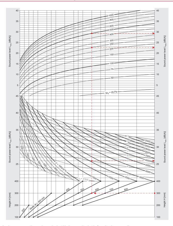
In the above nomogram, the sound power level outside the connecting duct is dimensioned as an overall level  $L_{WA}$ . Octave sound power levels  $L_{W-Oct}$  for every size and any required operating point are obtained from the WILDEBOER dimensioning software.
