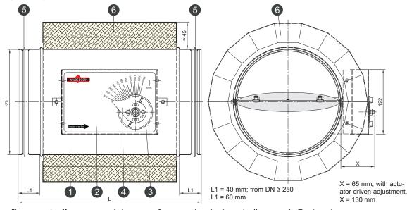
**VR1 volume flow controllers** are maintenance-free mechanical controllers that operate without an auxiliary power supply to maintain volume flows in ventilation and air conditioning systems constant.
