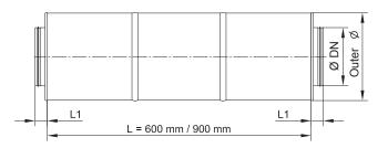
Maximum possible reduction of flow noise with sound attenuator lengths
