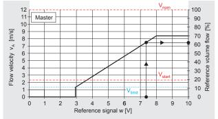
Master and Slave are set to 2 to 8 V in the "Variably adjustable" operation mode. The Master is set to  $V_{min}$  = 0%  $V_{nom}$  and  $V_{max}$  = 70%  $V_{nom}$  and controlled with w = 2 to 8 V.
