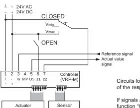
Circuits for override controls must be manufactured on site. Pay attention to mutual locking of the respective override controls (CLOSED,  $V_{min}$ ,  $V_{max}$ ) to avoid a short circuit!
