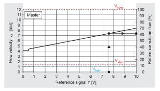
The operation modes "Variable 0 - 10 V" are set at the Master and Slave. The Master is then controlled with Y = 0 to 10 V.
