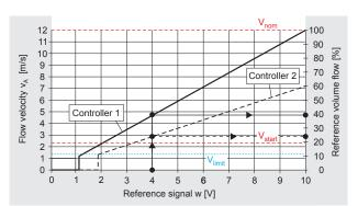
Stand-alone operation, parallel operation and Master/Slave sequential operation, examples (2)
