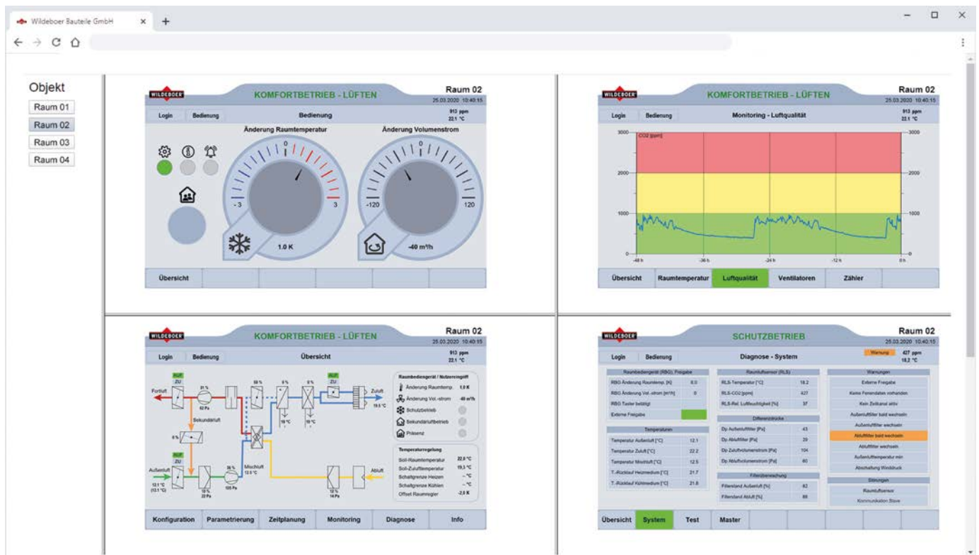
Example 5: Access to the ventilation units in one room, multiple different software views.
