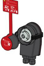
A protective film is fitted in the factory to protect the smoke switch and the protective screen from soiling during the construction stage. It must be removed before commissioning.
