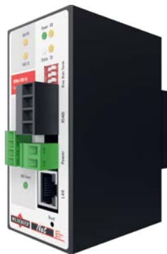
WiNet-GW-05 gateway WiNet-GW-06 gateway for BACnet, Modbus, OPC Server DA 2.0 and KNX
