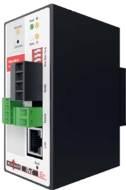
WiNet-GW-03 gateway WiNet-GW-04 gateway for BACnet, Modbus, OPC Server DA 2.0 and LON
