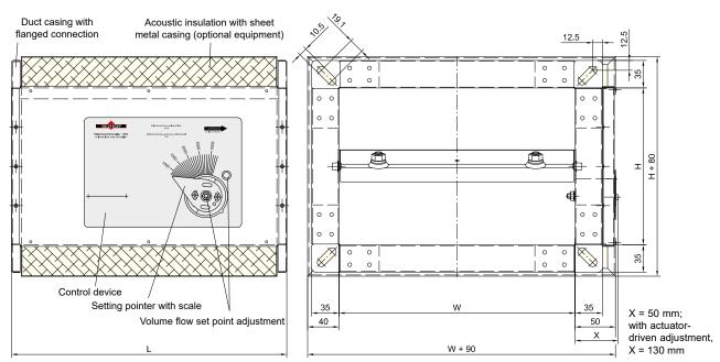
**VK2 volume flow controllers** are maintenance-free mechanical controllers that operate without any auxiliary power supply to maintain constant volume flows in ventilation and air conditioning systems.
